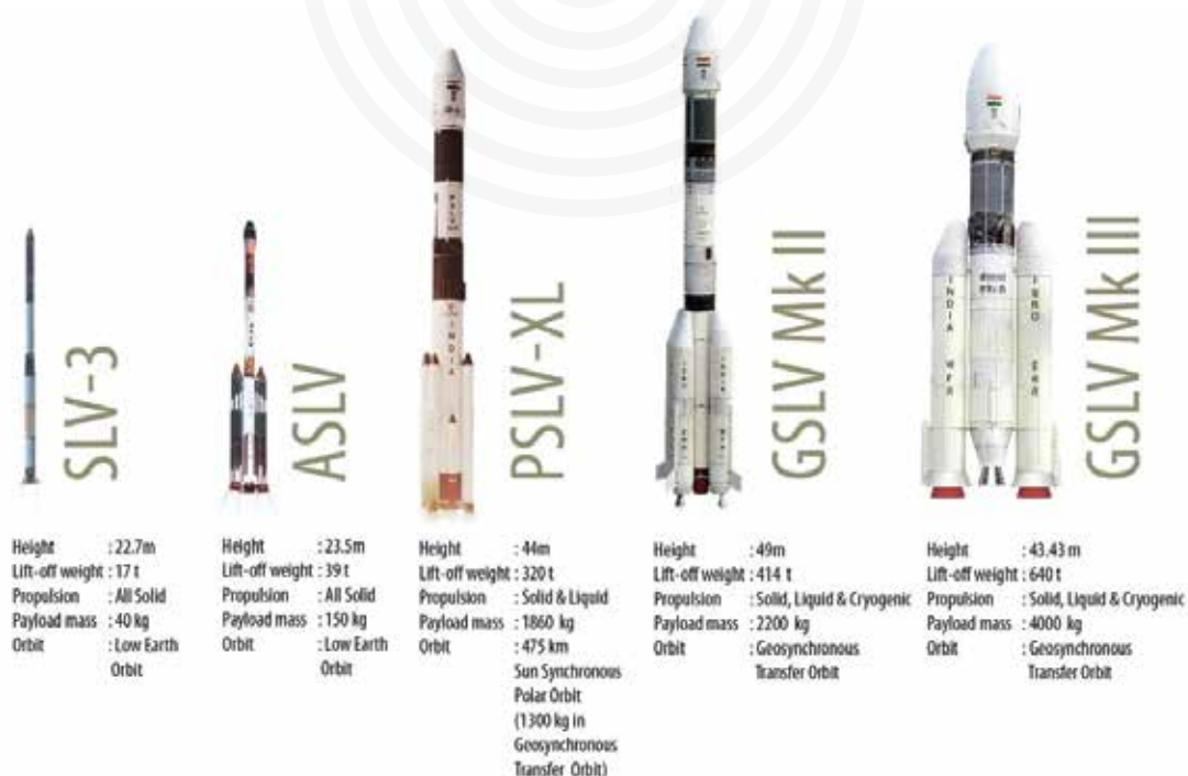
FIGURE: Polar Satellite Launch Vehicle (PSLV) was developed to launch Low-Earth Orbit (LEO) satellites into polar and sun synchronous orbits. Geosynchronous Satellite Launch Vehicle (GSLV) was developed to launch the heavier INSAT class of geosynchronous satellites into orbit.
